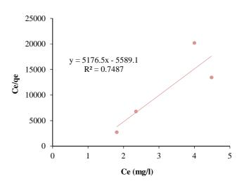
Figure 7. Curve of Langmuir adsorption isotherm
